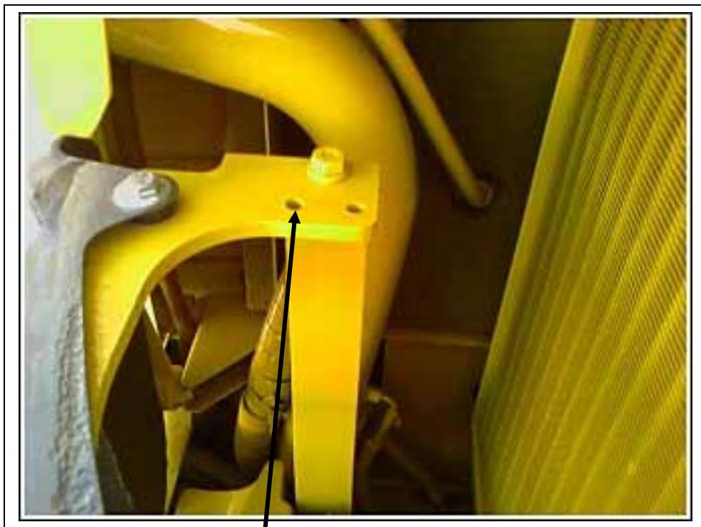
Mount 90° drier bracket off of threaded M10 bolt hole here.
