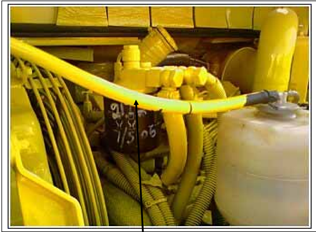
Fuel filter will be remounted to the A/C compressor mount to make room for the A/C compressor.
